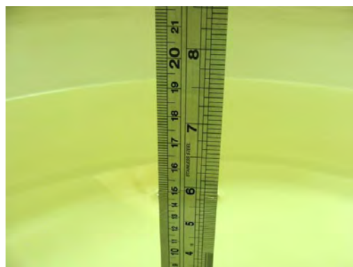
Fig 6.2 Photo of Liquid Height for Body SAR
