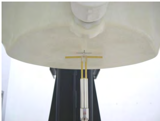
Fig 7.2 Photo of Dipole Setup
