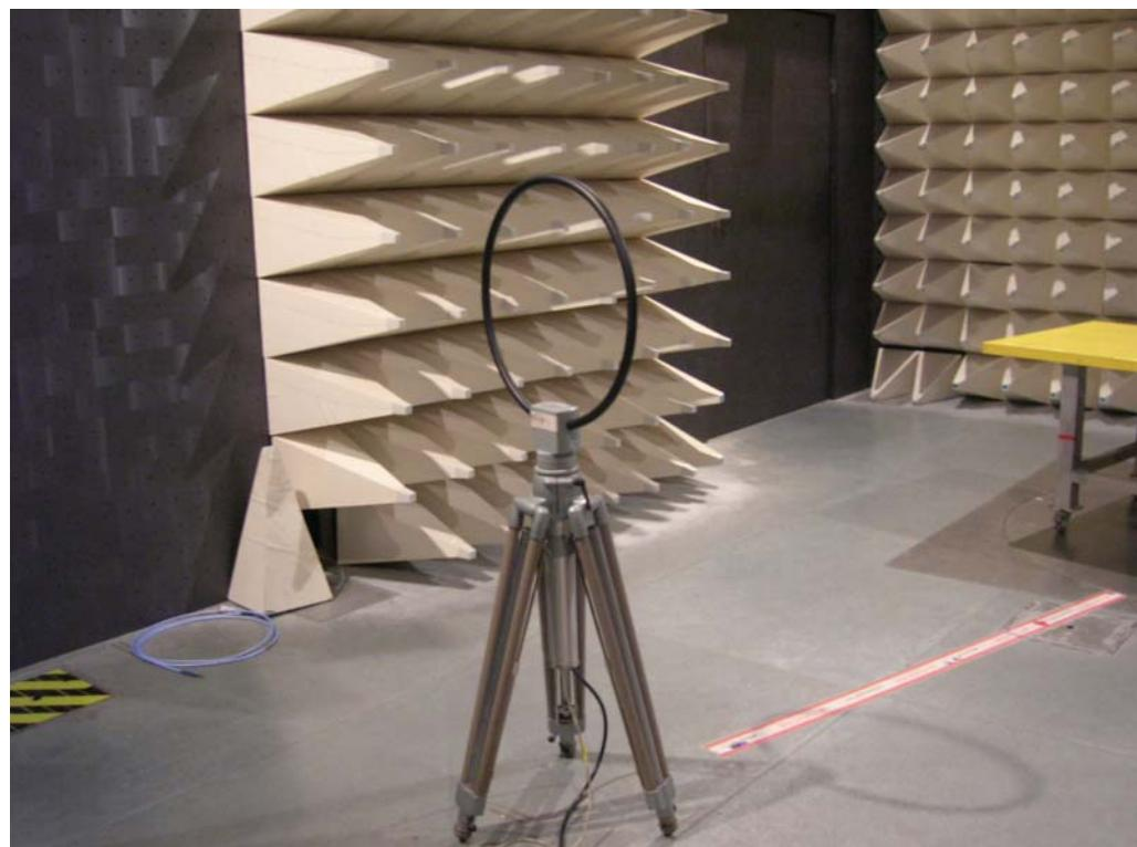
For radiated emissions 30MHz~1GHz
