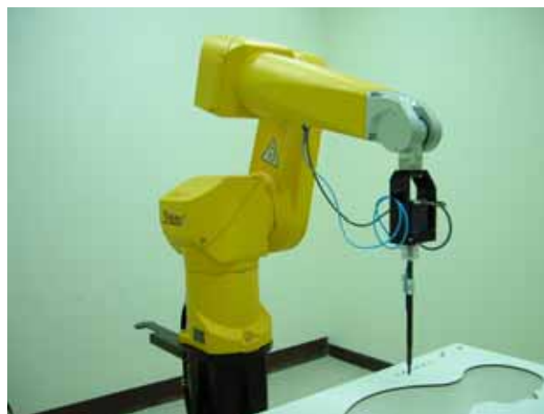
Fig. 5.2 Probe setup on robot
