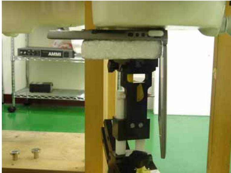
Fig. 9.1 Dell D400 Notebook Bottom Touch with Horizontal USB Port
