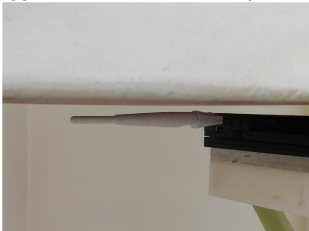
Horizontal Up, Test Separation 5 mm
