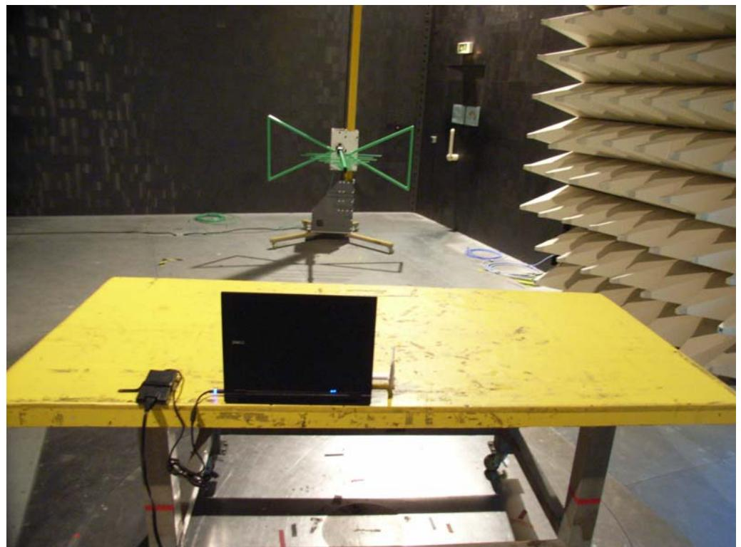
**For radiated emissions above 1GHz****FRONT VIEW**
