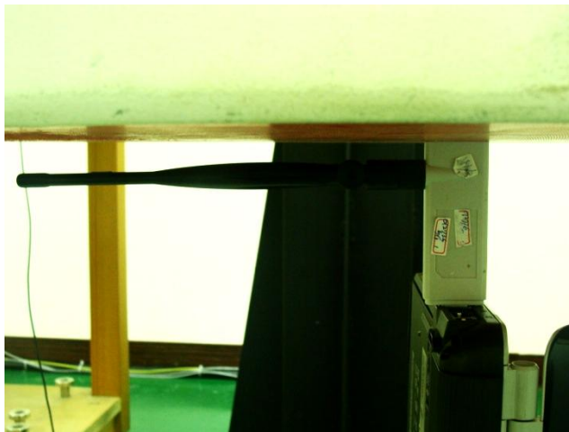
Direct Laptop Plug-in for Tip Mode (Tip Mode with Phantom 0 mm Gap) (Antenna is in Horizontal mode)
