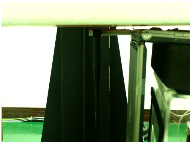
Direct Laptop Plug-in for USB Configuration 1 (Horizontal Up with Phantom 5 mm Gap) (Antenna is in Vertical mode)
