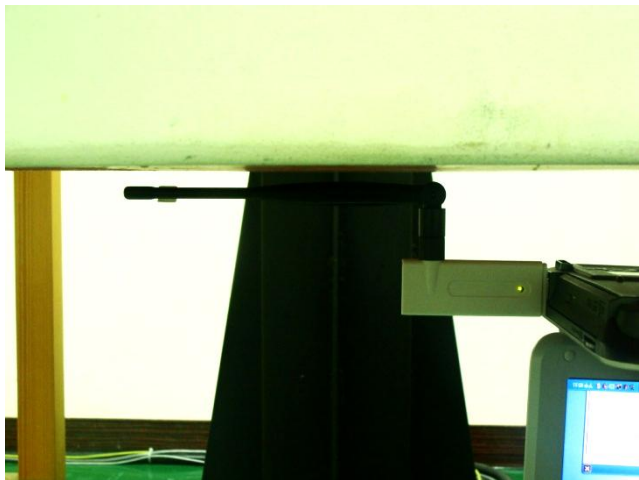
Direct Laptop Plug-in USB Configuration 4 (Vertical Back with Phantom 5 mm Gap) (Antenna is in Horizontal mode)
