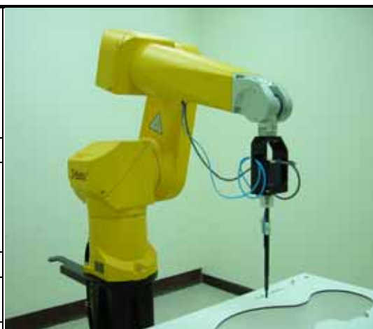
Fig. 5.2 Probe Setup on Robot
