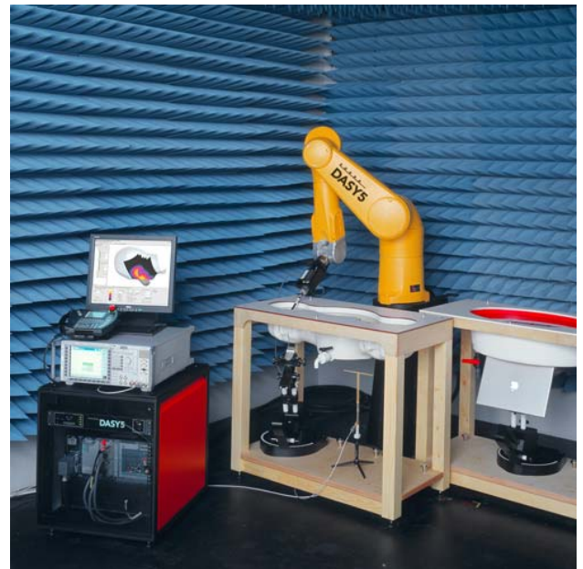
Fig. 5.2 Probe Setup on Robot
