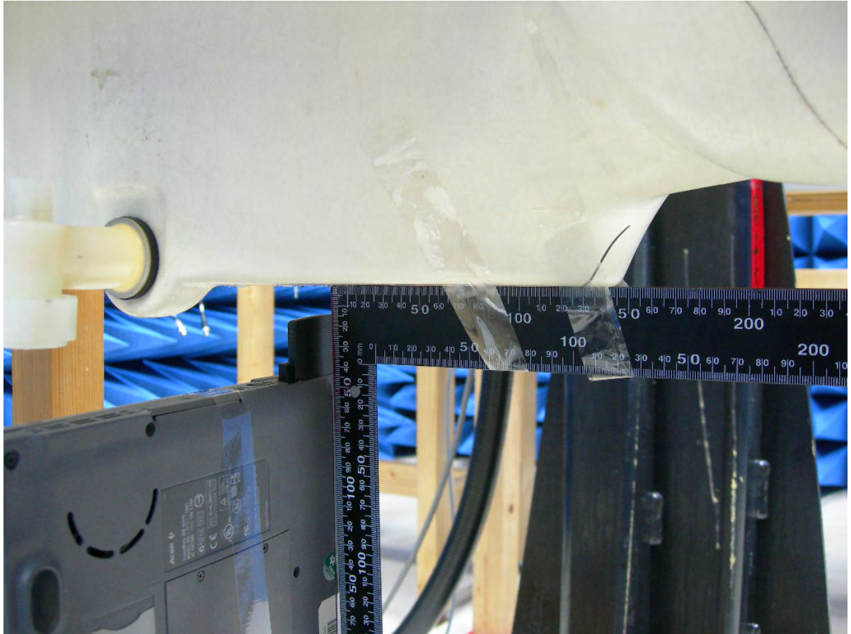
Figure 11.Body SAR Test Setup (Flat Section)_Tip
