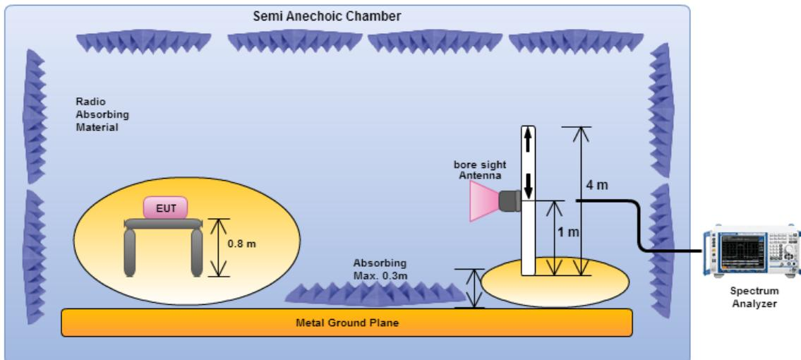
The frequency range of 1 GHz to 40 GHz using a calibrated horn antenna.
