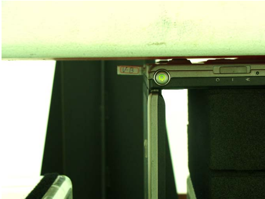
USB Configuration 1 (DUT Horizontal Up with Phantom 5 mm Gap)
