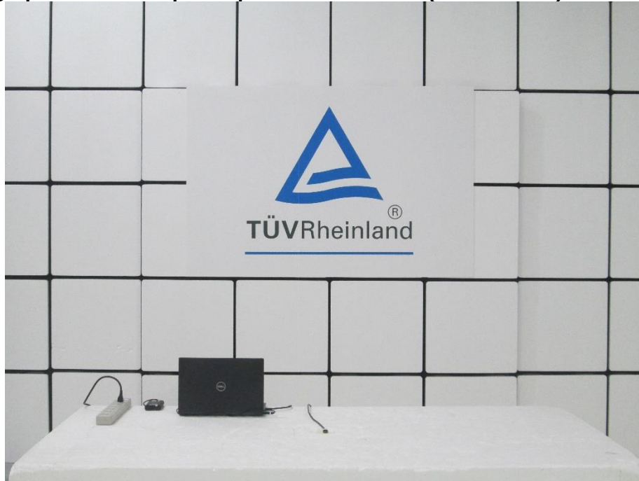
Photograph 2: Test Setup for Spurious Emissions (Front View 2)
