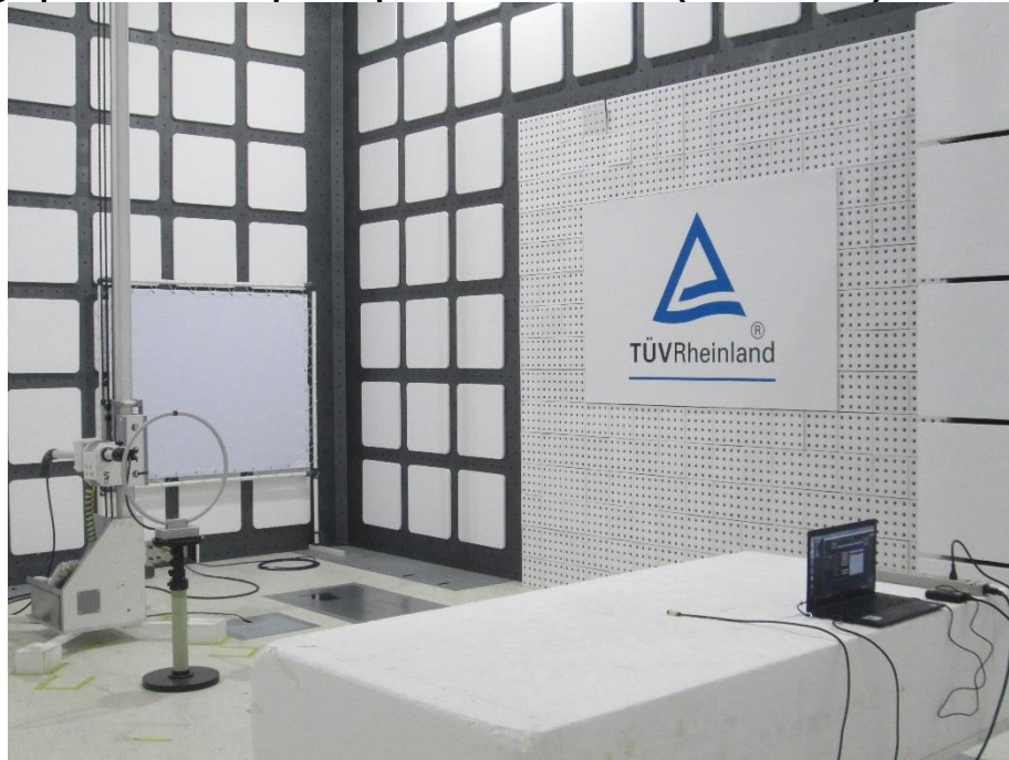
Photograph 4: Test Setup for Spurious Emissions (Back View 2)
