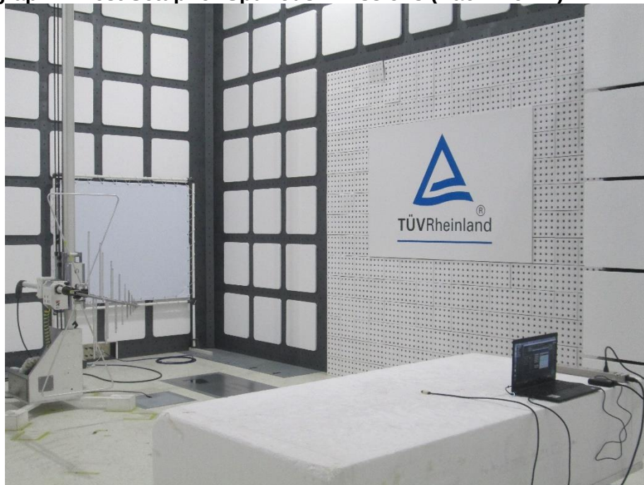
Photograph 4: Test Setup for Spurious Emissions (Back View 2)
