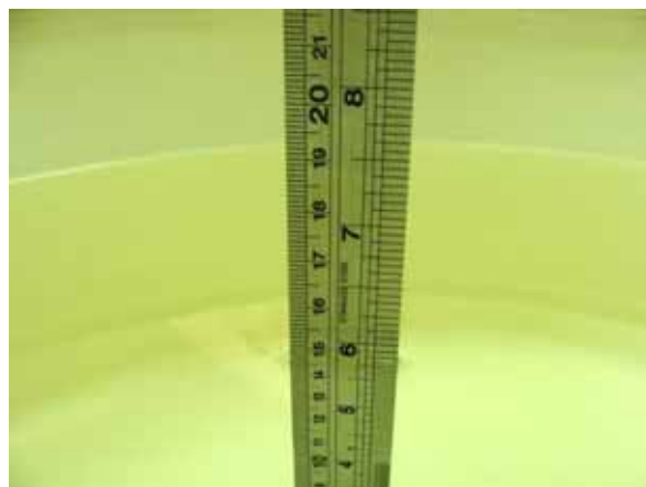
Fig 6.2 Photo of Liquid Height for Body SAR
