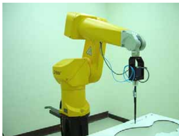
Fig. 5.2 Probe setup on robot
