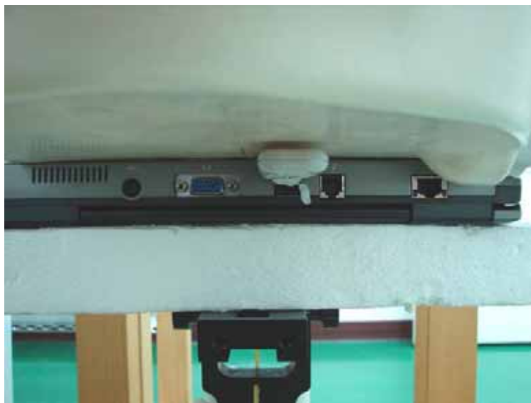
Fig. 9.1 Notebook Bottom Touch with Horizontal USB Port
