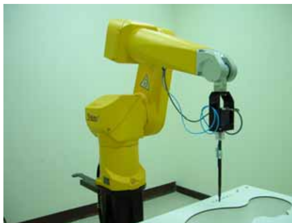
Fig. 5.2 Probe setup on robot
