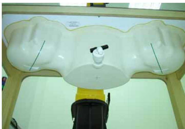
Fig. 5.4 Bottom view of twin phantom
