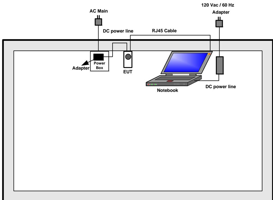
**Test Setup Diagram - Radiated Test Above 1GHz**
