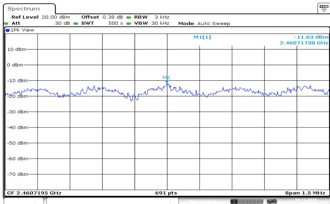
**IEEE 802.11n HT 40 MHz mode / Chain 0****PPSD (CH Low)**
