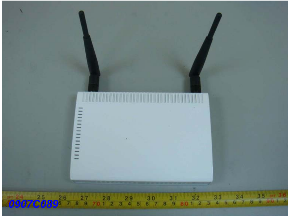
Photo No.: 13 Dipole Antenna: 2(Removable)
