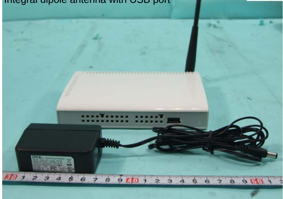
Integral dipole antenna with USB port
