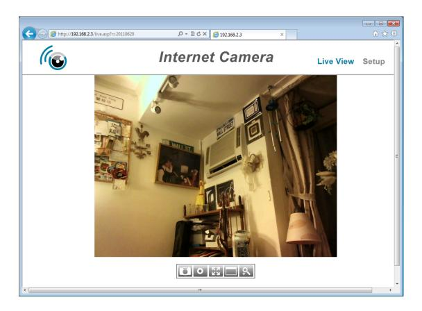
When you're in other setup pages of IP camera, you can click 'Live View' link located at the upper-right corner of IP camera's web interface:
