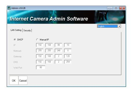
You can configure IP camera's IP address setting in this page. You can either use 'DHCP' (IP camera will acquire IP address from DHCP server on your local area network automatically), or 'Manual IP' (you have to input IP address manually).
