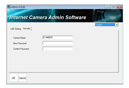
You can change IP camera's name, and change its administrator password here by inputting new password in both 'New Password' and 'Confirm Password' field.
