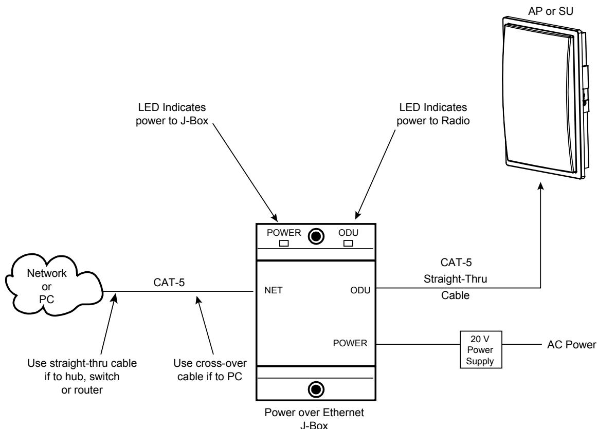
Both green LED's on the J-box should be lit, indicating power is present at the J-box as well as the radio. You are now ready to configure the radio via the Ethernet port.
