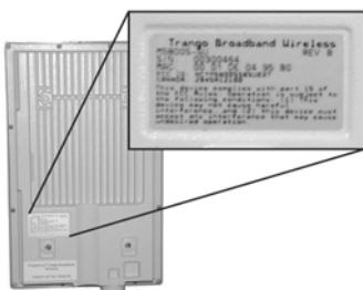
APs and SUs look identical. The only way to tell them apart is by the model number printed on the backside product label. This label also contains the MAC ID of the radio as well as the serial #.
