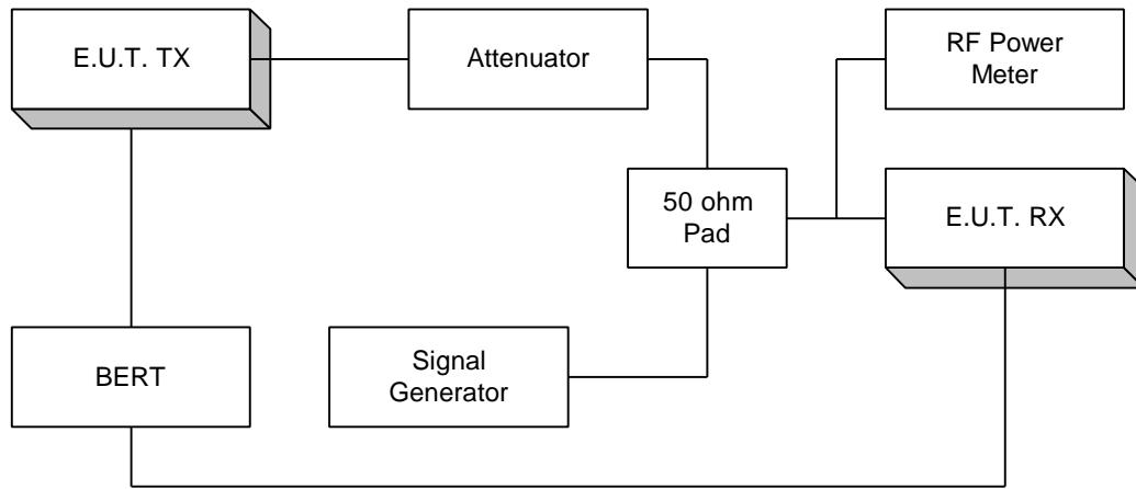
**NOTE:** This is a typical setup. The setup may vary slightly since many devices have BER test functions built into the device.
