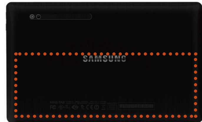
The location of the internal battery
