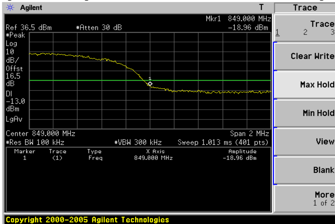
Figure 8-20: Band edge emission at antenna terminals –WCDMA V Channel Highest
