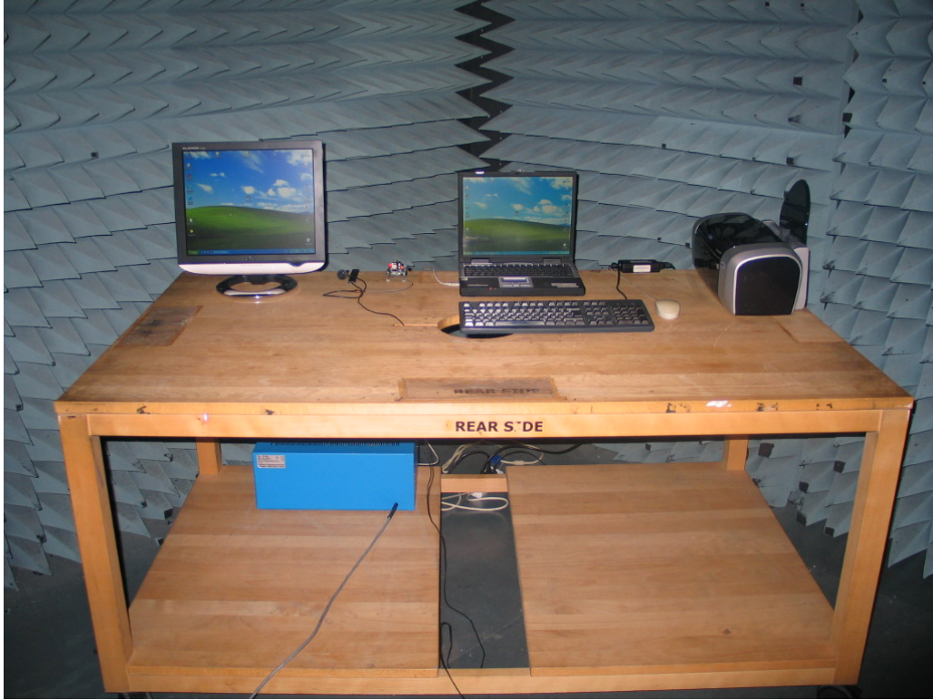
Photo 1: Test setup for radiated measurements
