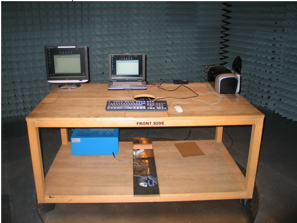
Photo 2: Test setup for radiated measurements
