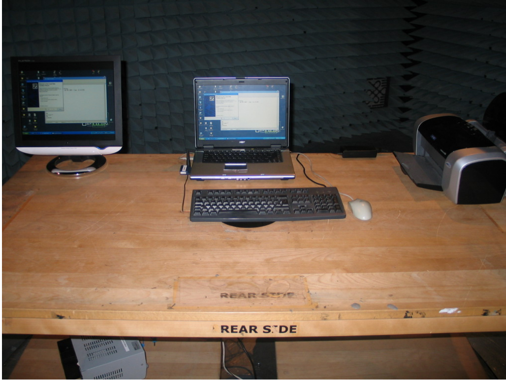
Photo 1: Test setup for radiated measurements
