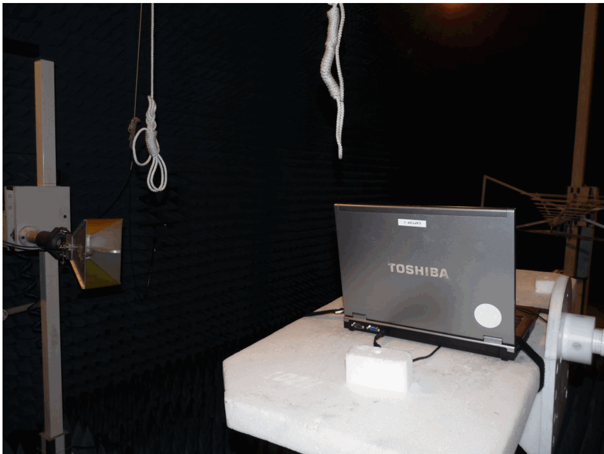
test set-up for radiated measurements
