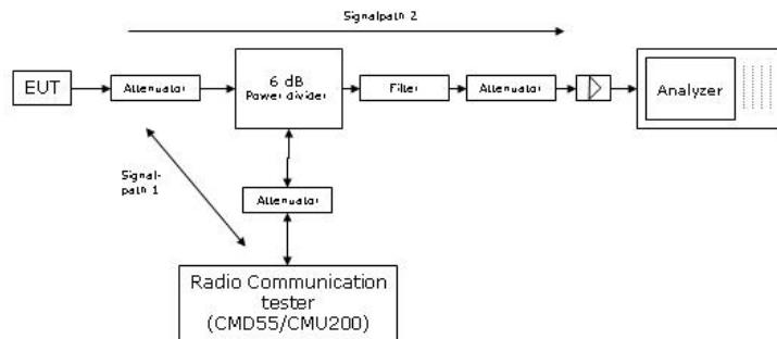
Remark: Depending on the frequency range suitable attenuators and/or filters and/or amplifiers are used.
