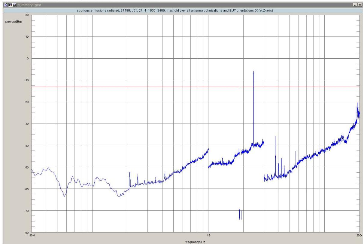
**Test: 24.4; Frequency Band = FDD2, Mode = HSDPA, Channel = 9400, Frequency = 1880MHz**
