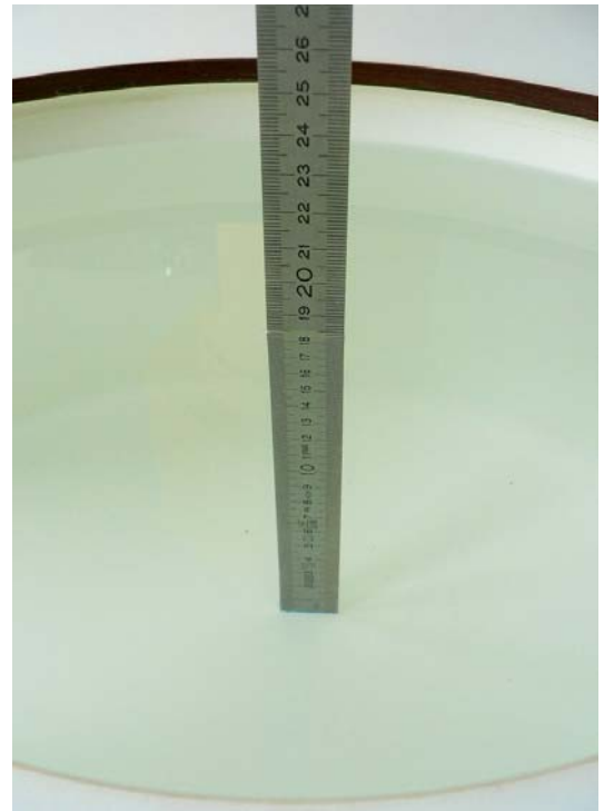
Fig. 28: Liquid depth for GPRS/EDGE 1900 and WCDMA II Body measurements.
