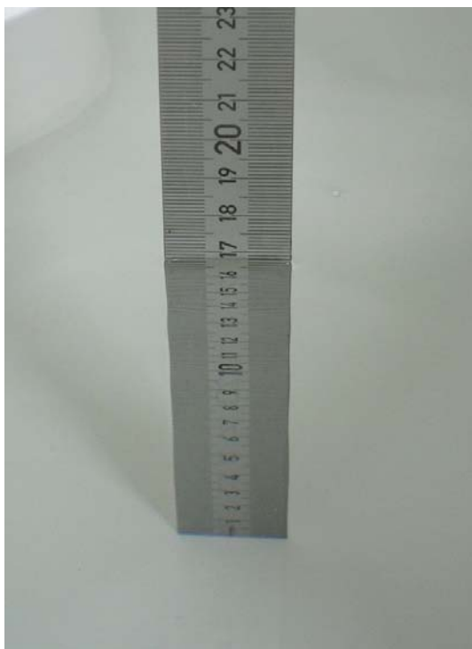
Fig. 29: Liquid depth for IEEE 802.11 Body measurements
