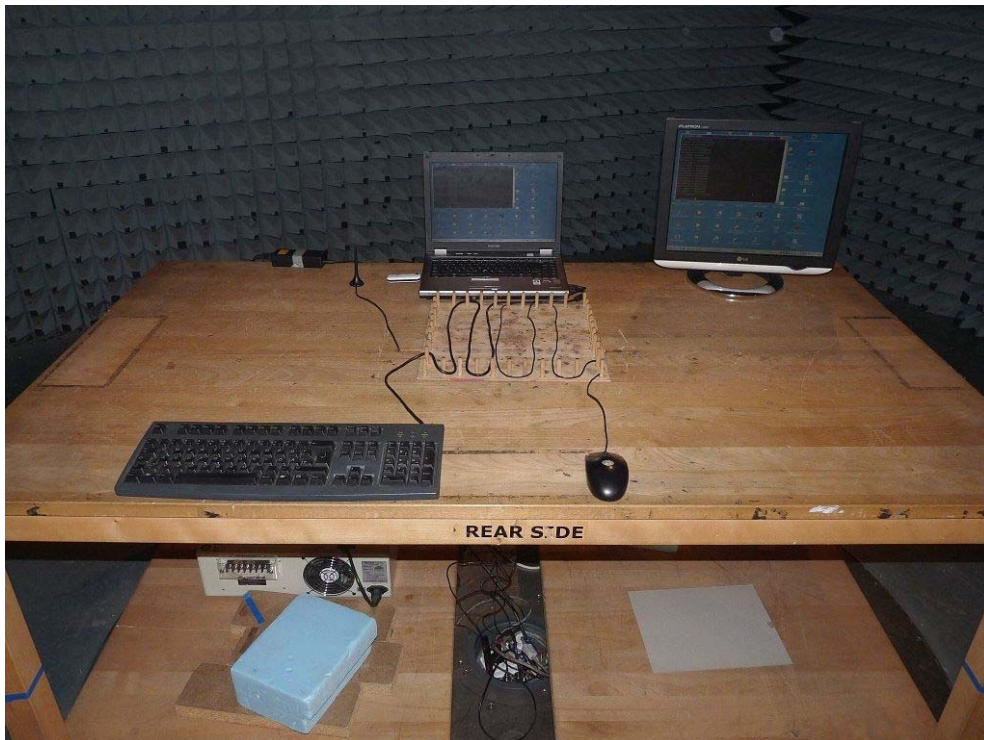
Photo 5: Test setup for radiated measurements (emission measurement using computer periphery setup)
