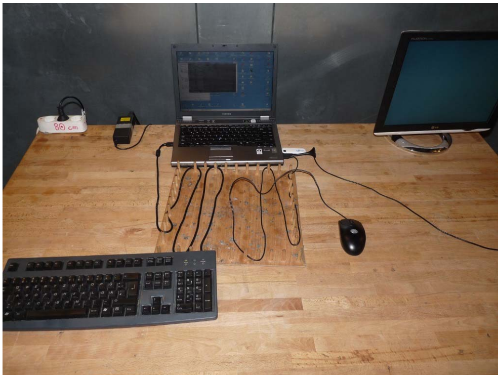
Photo 6: Test setup for conducted measurements (AC Port (power line) using computer periphery setup)
