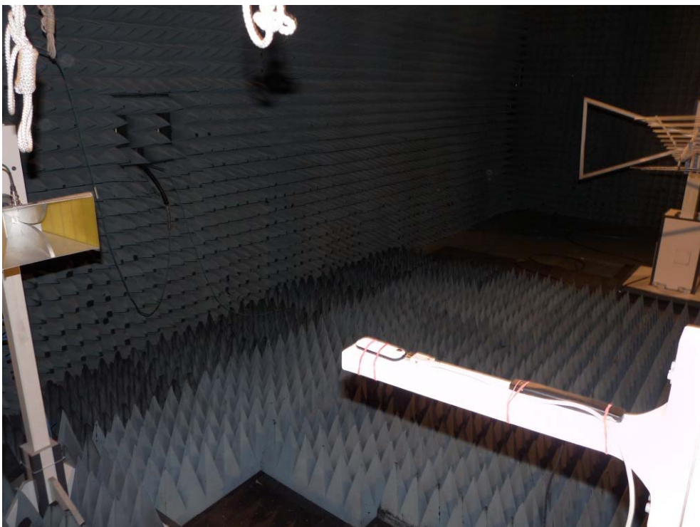
Photo 4: Test setup for radiated measurements (Enclosure, radiated output power measurement)
