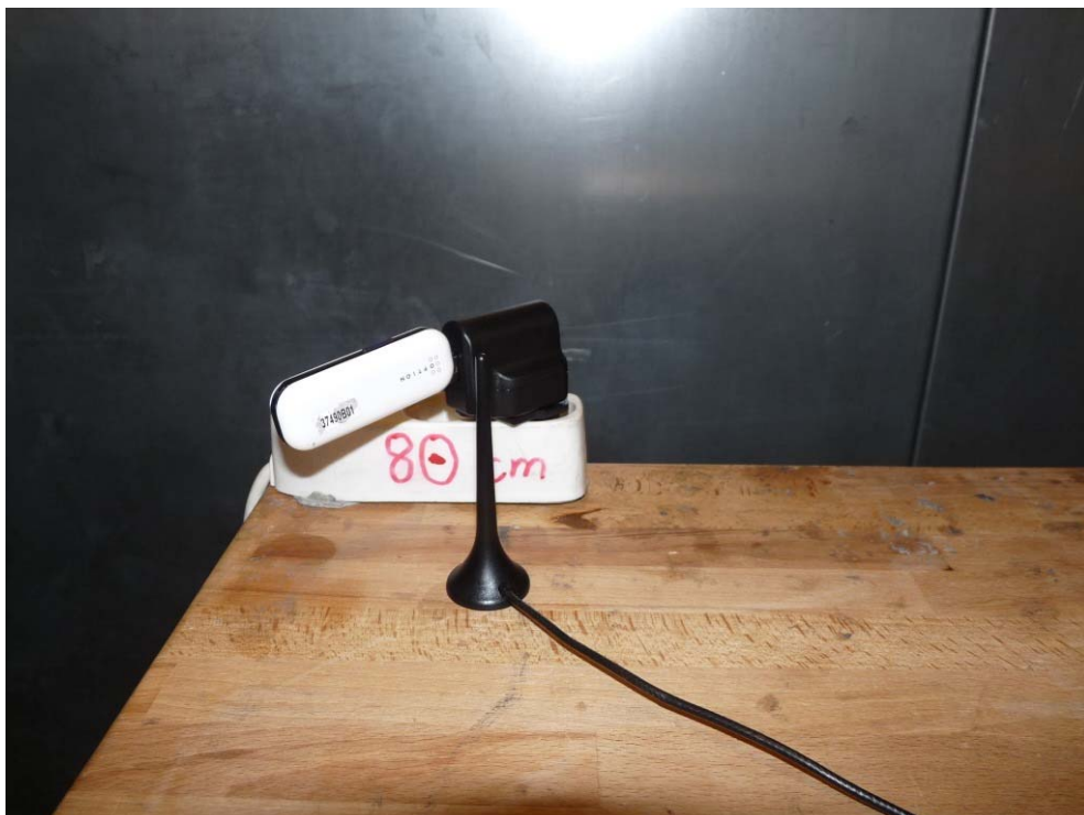
Photo 7: Test setup for conducted measurements (AC Port (power line))
