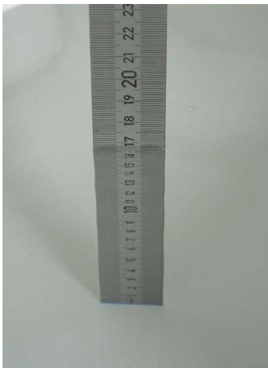
Fig. 29: Liquid depth for IEEE 802.11 Body measurements
