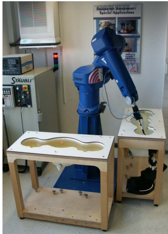
Fig. 4: The measurement set-up with two SAM phantoms containing tissue simulating liquid.
