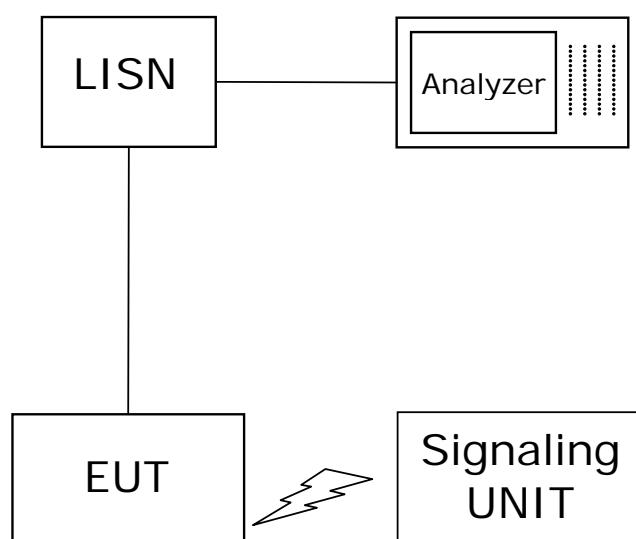
Setup in the shielded room for conducted measurements at AC mains port
