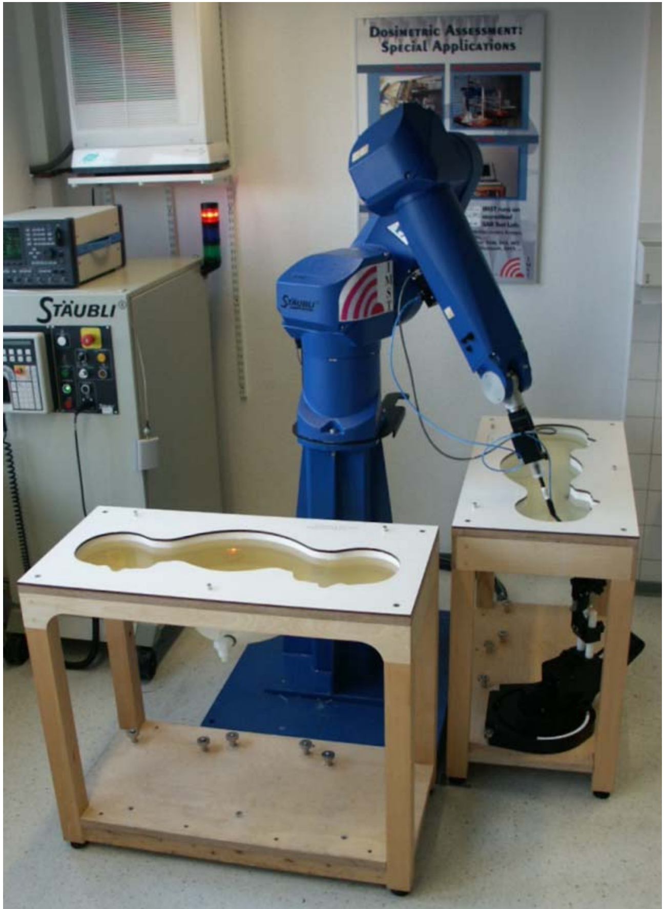
Fig. 5: The measurement set-up with two SAM phantoms containing tissue simulating liquid.
