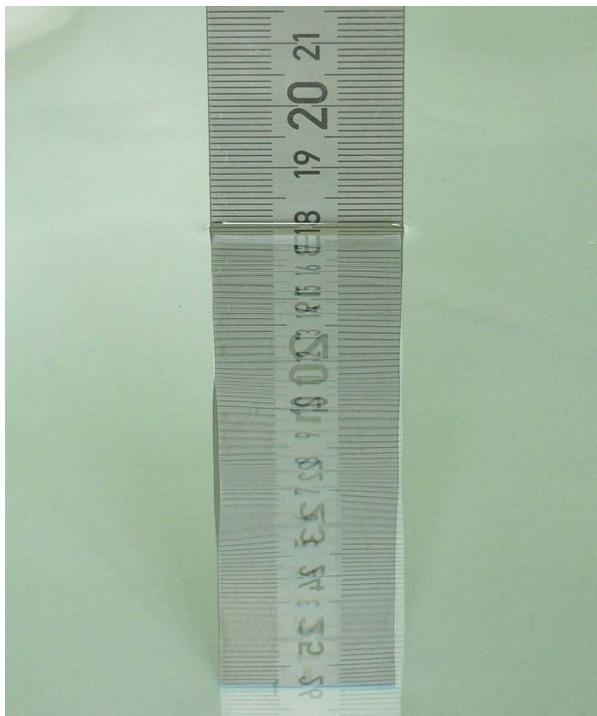
Fig. 24: Liquid depth for WCDMA IV Body measurements
