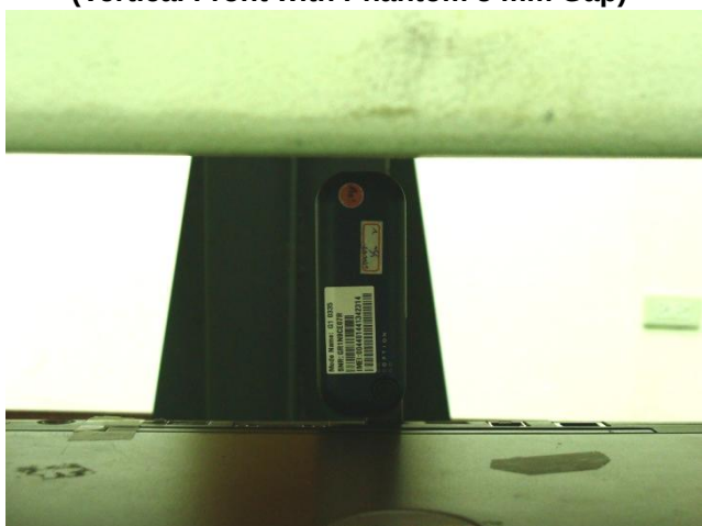
Direct Laptop Plug-in for USB Tip Mode (Tip of Dongle with Phantom 5 mm Gap)
