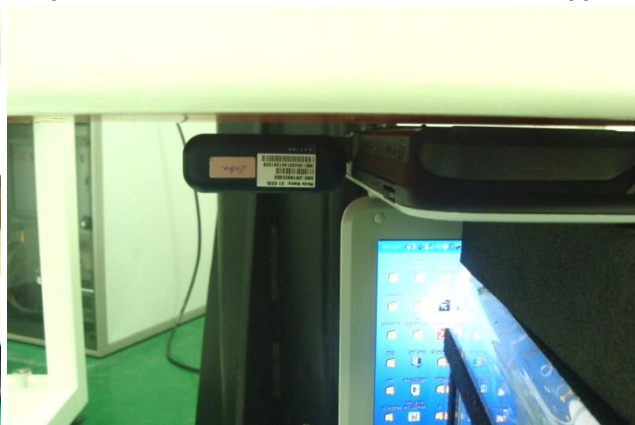
Direct Laptop Plug-in USB Configuration 4 (Vertical Back with Phantom 5 mm Gap)
