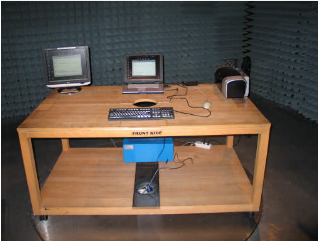
Photo 1: Test setup for radiated measurements
