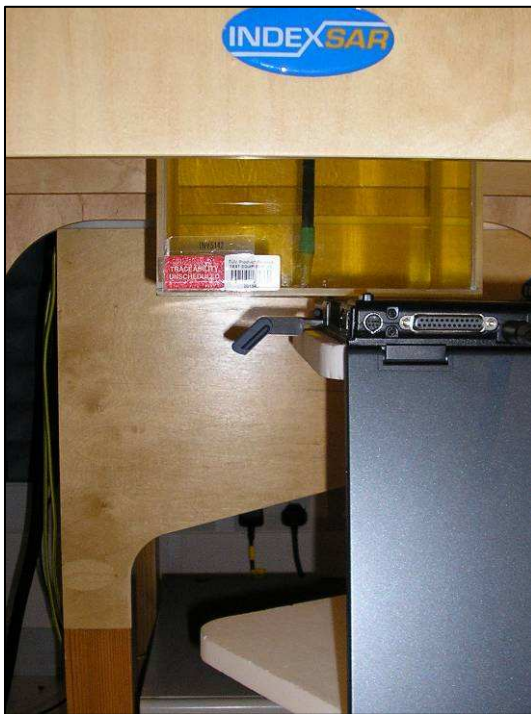
Figure 12: Front Positional Photograph of the Option nv GE0301 Express Card in 11mm Separation distance configuration from the bottom of the flat phantom (Host laptop used: HP Compaq nc 6320 – in touch position) FDD Band V testing (850MHz Body fluid shown)
