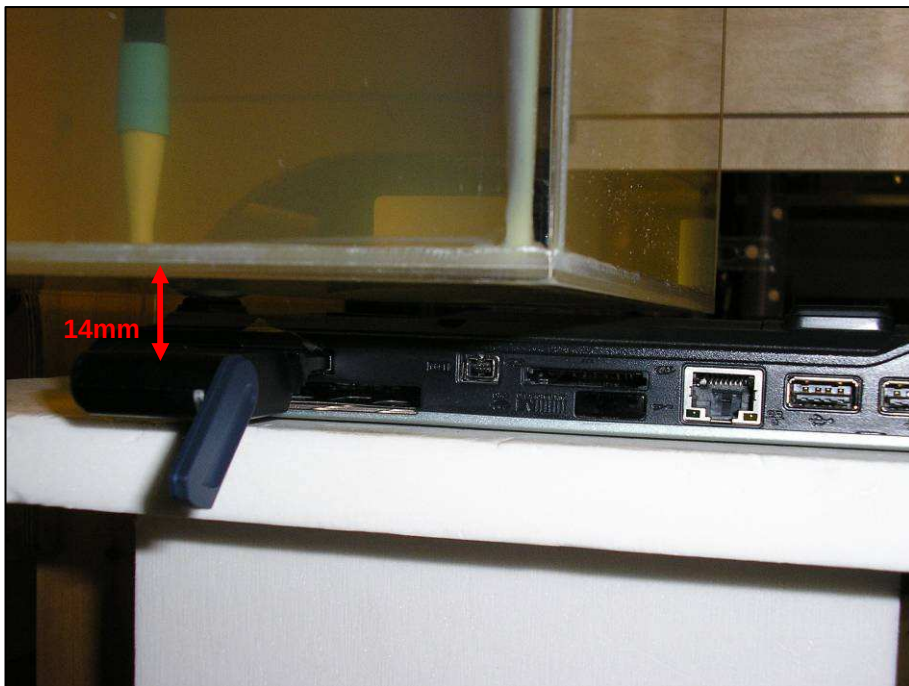
Figure 11: Side Positional Photograph of the Option nv GE0301 Express Card in 14mm Separation distance configuration from the bottom of the flat phantom (Host laptop used: Acer TravelMate 4260 Series – in touch position) FDD Band II testing (1900MHz Body fluid shown)
