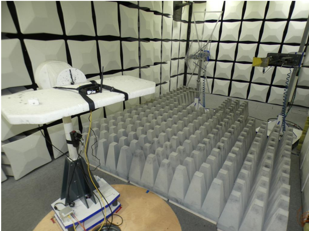
Photo 3: Test setup for radiated measurements above 1 GHz (FAC)
