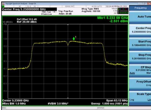
U-NII-3 Power spectral density-802.11 n(20MHz),5745MHz
