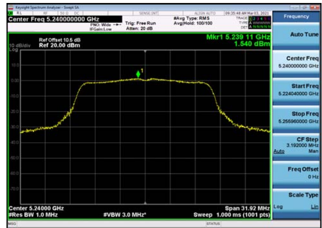
U-NII-1 Power spectral density-802.11 ac(20MHz),5220MHz
