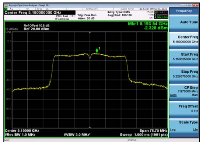
U-NII-1 Power spectral density-802.11 a(20MHz),5180MHz
