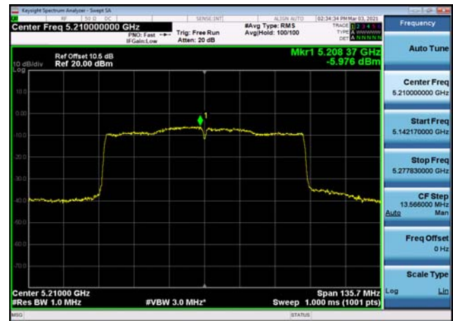
U-NII-3 Power spectral density-802.11 n(20MHz),5785MHz
