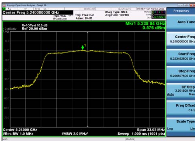
U-NII-1 Power spectral density-802.11 n(40MHz),5230MHz
