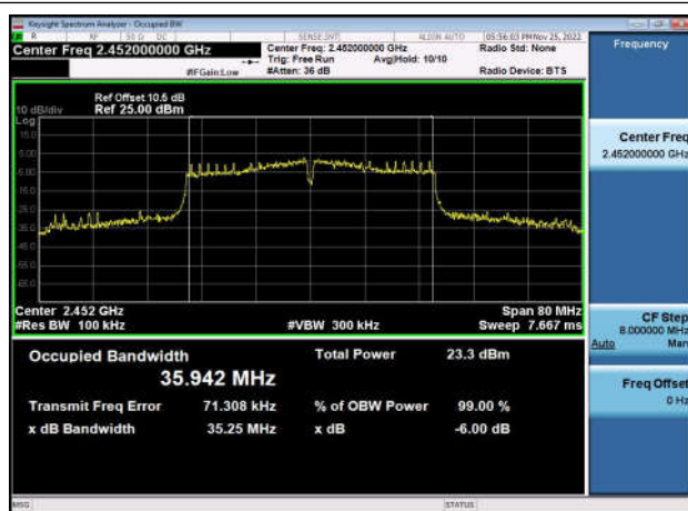
6dB Bandwidth-802.11n(HT40),2452MHz , Ant0
