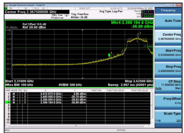
,Plot 2,Band Edge-802.11g,2462MHz ,Ant0
