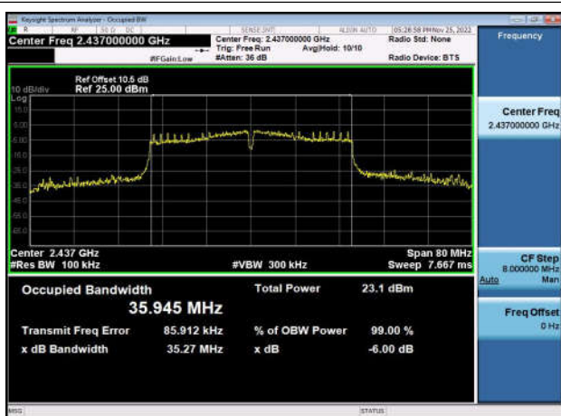
6dB Bandwidth-802.11n(HT40),2437MHz , Ant0
