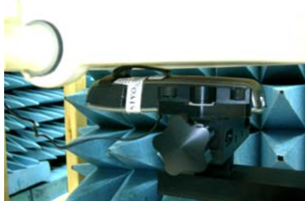
Figure 18. Body SAR Test Setup (Flat Section)
