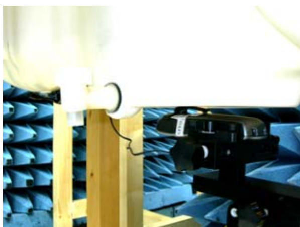
Figure 17. Body SAR Test Setup (Flat Section)
