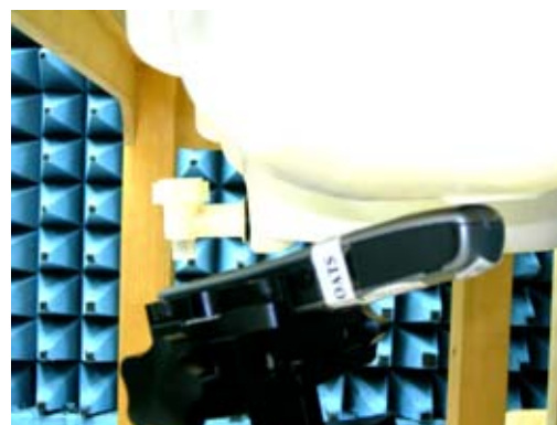
Figure 16. Left Head SAR Test Setup (Tilted)
