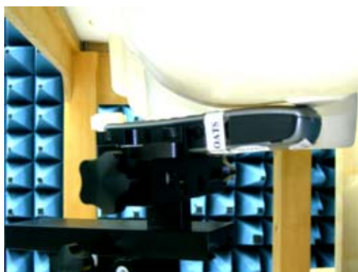
Figure 15. Left Head SAR Test Setup (Cheek)
