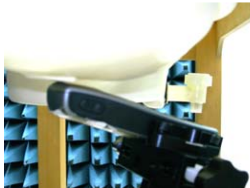
Figure 14. Right Head SAR Test Setup (Tilted)
