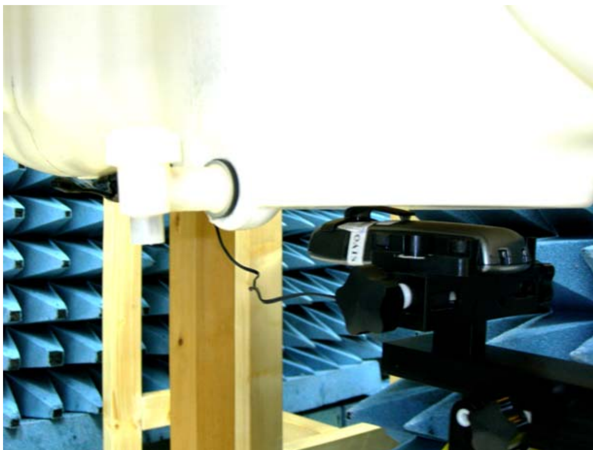
Figure 25. Body SAR Test Setup (Flat Section)
