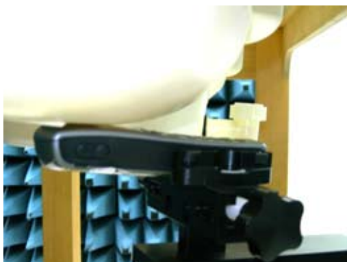
Figure 13. Right Head SAR Test Setup (Cheek)
