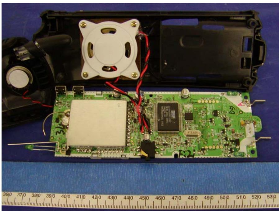
**EUT - Main Board Component View without Shielding**
