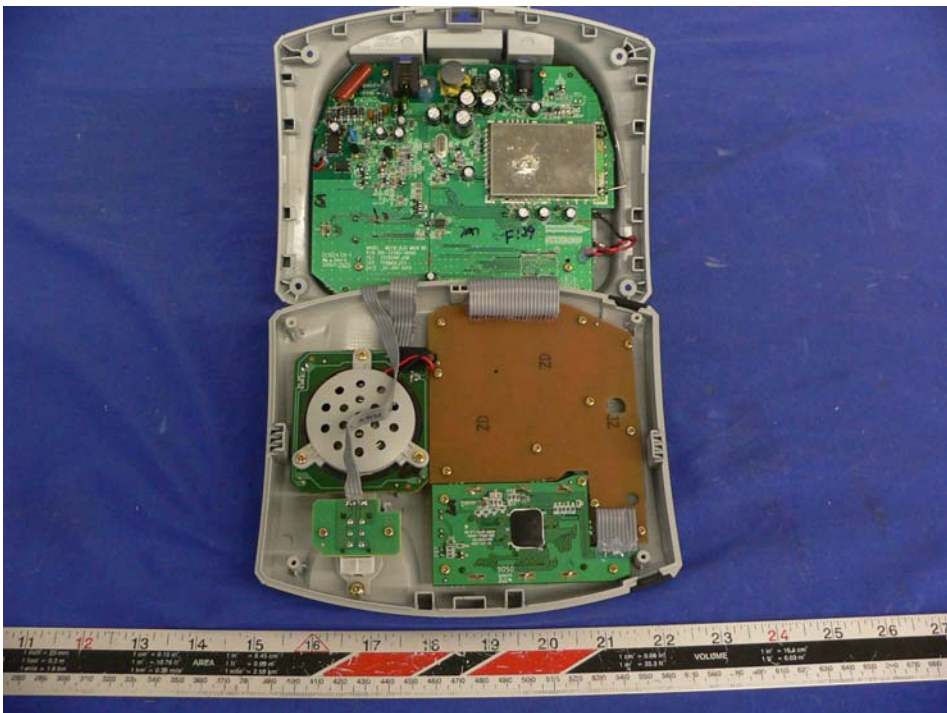
EUT - Main Board Solder View
