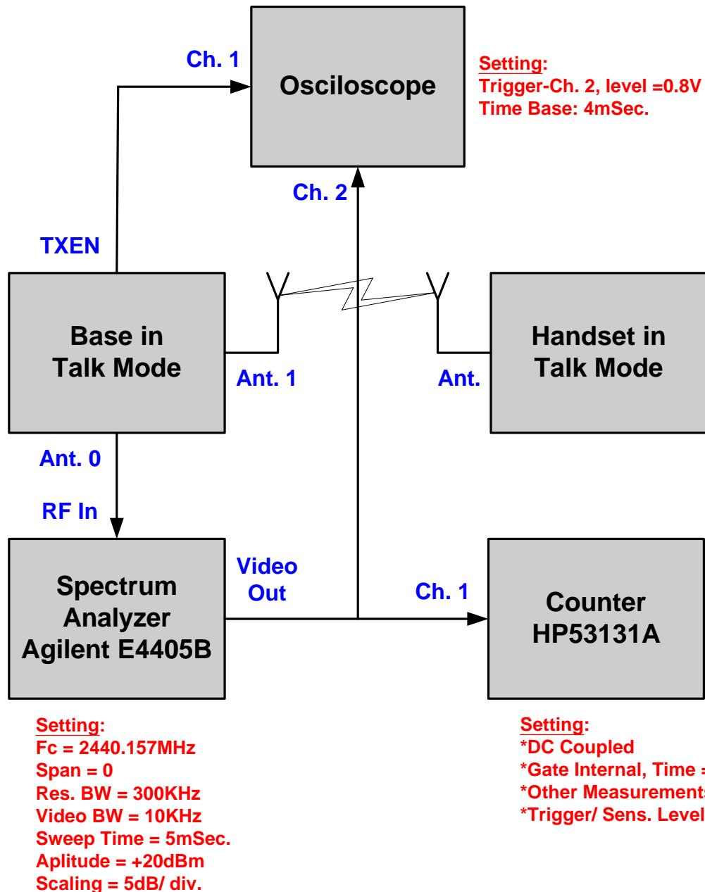
Step 1: Establish Single Channel “Talk mode” BS/HS Link on Ch55. Note SA Video output level on Scope for both Antenna Selections. Repeat for Adjacent Channels – See Plot 7. Note that a “pulse threshold” = 1.2V clearly indicates a Ch55 “hit”.
