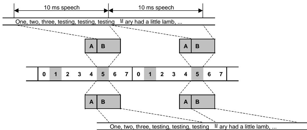
The following diagram shows a dummy bearer transmission. Note, that it uses only a down-link slot and the A-field of the packet.
