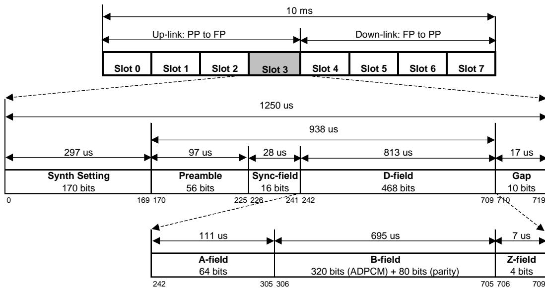
The basic, repeating, frame structure is 10 ms long. It is sub-divided into 8 slots, each 1250 µs long. The active transmission time is 937.5 µs. The first 4 slots form the 'up-link', when the PPs transmit to the FP. The last 4 slots form the 'down-link', when the FP transmits to the PPs.
