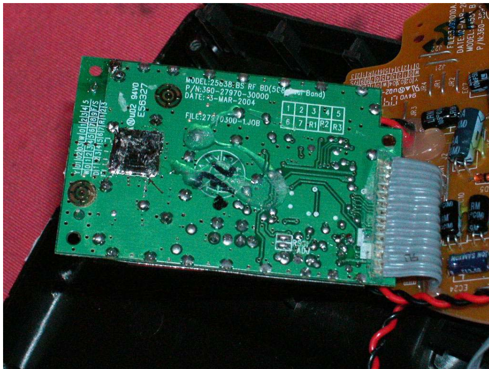
Base Oscillator PCB solder side
