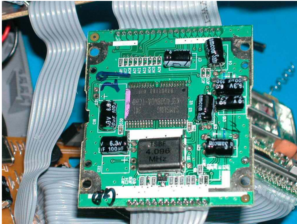
Base Answering Machine MCU PCB rear side
