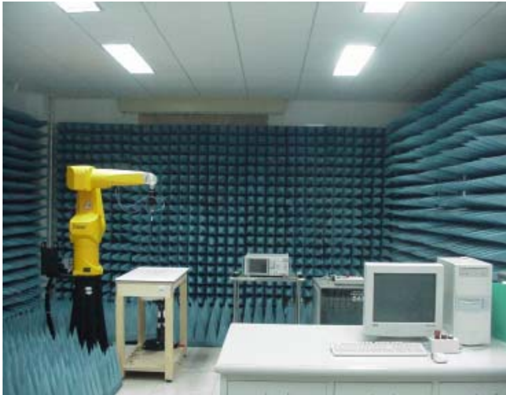
Picture 1 Specific Absorption Rate Test Layout
