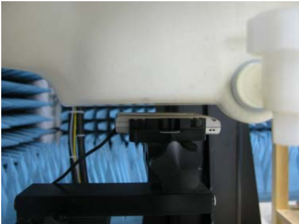
Picture 6 Flat Phantom -- Body-worn Position (the distance from handset to the bottom of the Phantom is 1.5cm)
