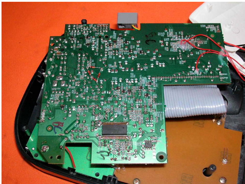
Base Main PCB solder side
